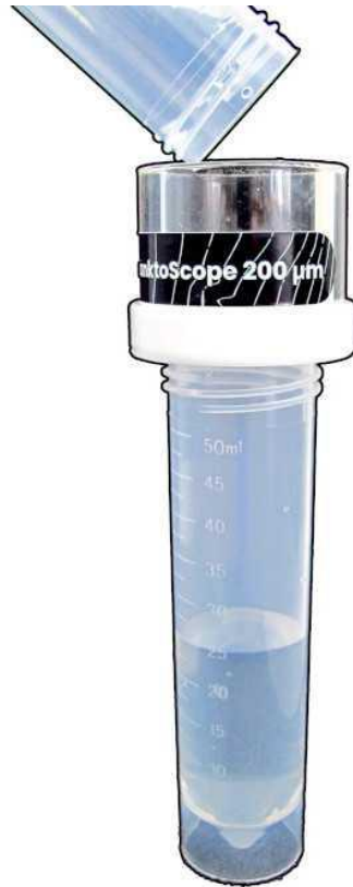
Figure 1: How to filter the sample with the 200 \mu\text{m} sieve
